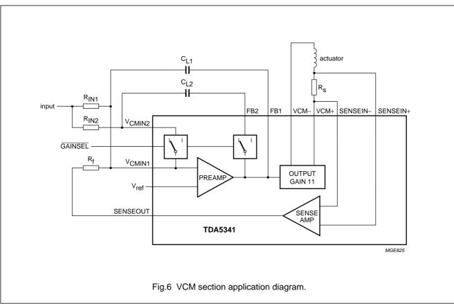
$$T = -11 \times R_{f} \times Z_{L} \times \left(\frac{1}{R_{IN} \times (R_{f} \times R_{s} + R_{f} \times Z_{VCM} + 110 \times R_{s} \times Z_{L})}\right)$$
